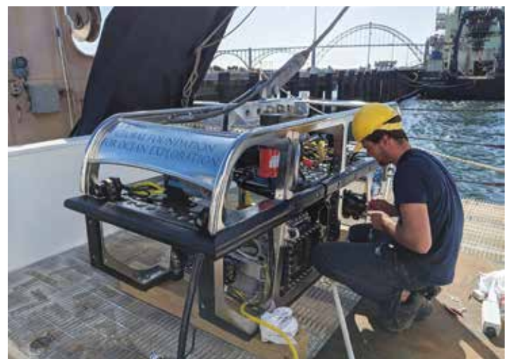
EXPRESS partners deployed Yogi and Guru , a two-body ROV system, from NOAA R/V Reuben Lasker during a fall 2019 cruise to survey deep-sea corals, sponges and fish habitat off the U.S. West Coast. Operating in tandem, Yogi worked along the bottom of the ocean collecting samples, high-resolution video and still images while Guru , a camera and lighting sled, hovered above allowing pilots to maintain visual contact with Yogi below. Both vehicles sent all data they collected back to the ship via a fiberoptic tether. Yogi photo provided courtesy of Daniel R. Rogers. GURU photo provided courtesy of Josh Carlson, GFOE.
