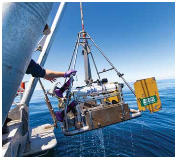
USGS SEABOSS is built specifically for sampling and photographing seabed features for sediment monitoring. Photo by contractor Steve De Neef.
