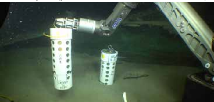
Placement of biofilm recruitment experiments near a shipwreck during the 2014 GOM-SCHEMA study. Photo by Deep Sea Systems International's Global Explorer ROV.
