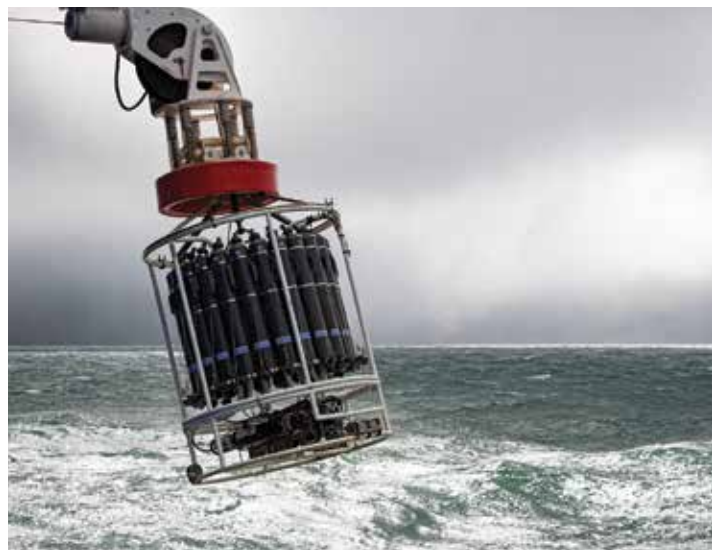
Niskin water sampling rosette deployment on board the R/V Sikuliaq . Photo provided by Brendan Smith, North Pacific Research Board Arctic Program.
